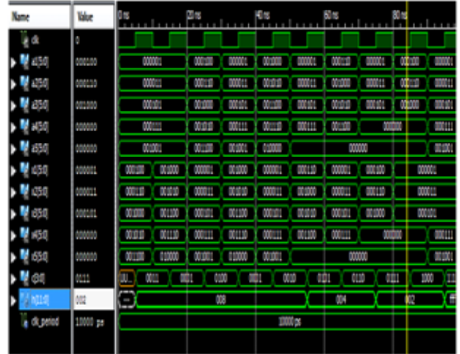
Fig.4. Timing diagram of MAX-MIN Calculator.
