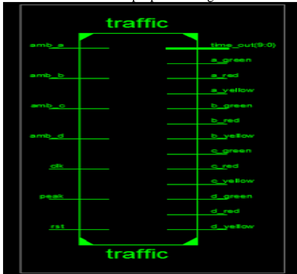
Fig.2. The block diagram of Real-Time Traffic Light controller system after synthesis.
