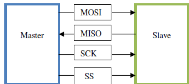
Fig.1. Master/Slave block diagram of SPI.
